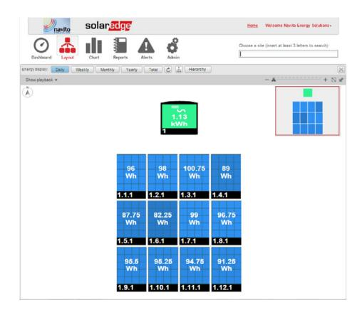
The web-based SolarEdge monitoring portal provides enhanced PV performance monitoring and yield assurance through immediate fault detection and alerts at module level, string level and system level.
